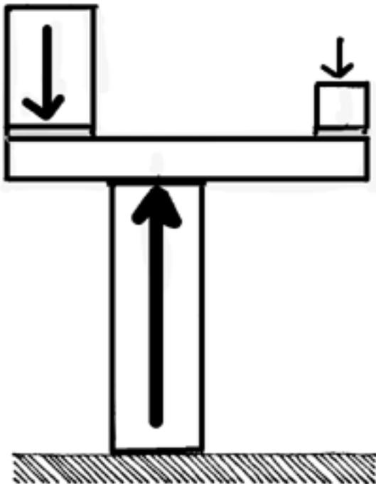
**Fig. 6.** Balancing compressive loads.
