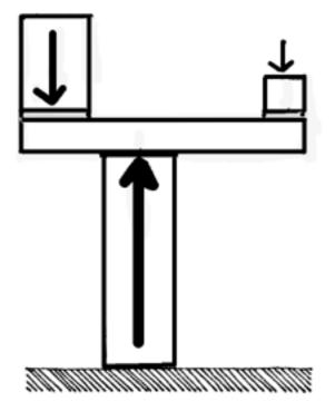
Fig. 6. Balancing compressive loads.
