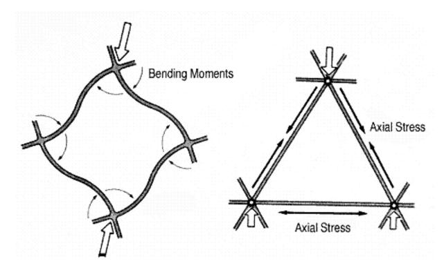
Fig. 7. Loading a square and loading a triangular truss.
